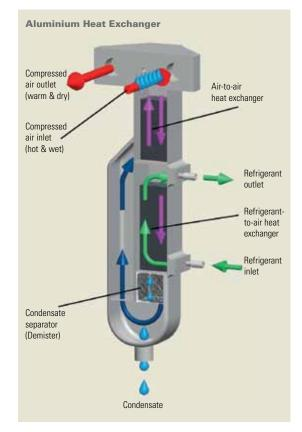
The main feature of the Buran refrigeration compressed air dryer is the aluminium heat exchanger  $% \left( {{{\rm{T}}_{{\rm{T}}}}_{{\rm{T}}}} \right)$
