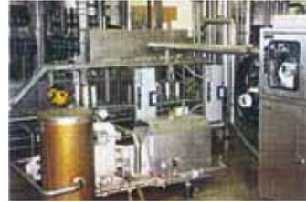
Finally, in the afterfilter, remaining particles from the drying agent are retained.
